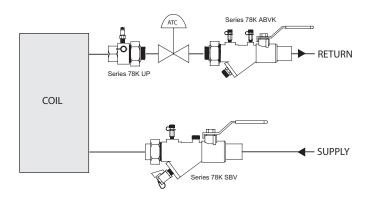
The TA Series 78K Automatic Balance Koil-Kit<sup>®</sup> provides a simplified, quality coil circuit installation while ensuring optimal hydronic system design requirements are met. Suitable for hot, cold, treated and untreated systems, the Automatic Balance Koil-Kit<sup>®</sup> is a reliable 3-component package featuring:
