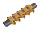
Style 155 Expansion Joints are a combination of couplings and specially machined pipe nipples, joined in series to accommodate piping system expansion/contraction.
