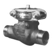
Available with Type 316 stainless body and trim in the 2" (50 mm) size, Swinger check valves are supplied with bonnet cap drilled and tapped with 1/2" (12.7 mm) NPT pipe plug for chemical injection or other auxiliary connections.
