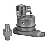
Series 767 introduces a new concept in actuator design, featuring a single trip point for the pneumatic event, regardless of supply water pressure, and an integral electric solenoid. The Series 767 Electric/ Pneumatic Double Interlock low pressure actuator is designed to trigger systems using the Series 769 FireLock NXT Preaction valve, per 30.82. This new design allows you to set the system without having to activate the solenoid.
