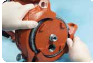
Remove coupling and closure cap
