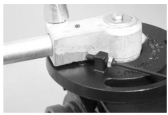
**19.** Open the valve until the pointer aligns with the "OPEN" marking. Turn the remaining travel limit's socket set screw until it contacts the side of the handle's hub.
