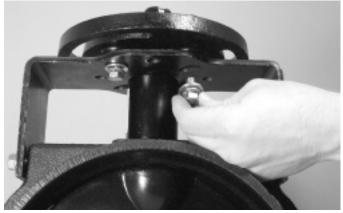
7. Place one %-inch lock washer and one %-inch flat washer onto each of the four hex-head screws (%-16 UNC X %" long). Install these screws up through the valve bracket and into the tapped bosses of the dial stop plate until they are hand tight.
