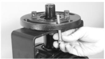
**9.** Insert the % –16  $\times$  3" long carriage bolt up through the bottom of the dial plate. Slide the carriage bolt in toward the bracket so that the head of the bolt rests on the top of the bracket.
