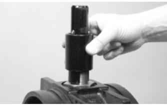
4. Install the stem adapter sleeve over the stem adapter.
