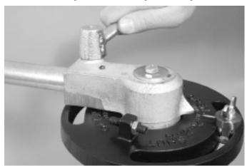
**3.** When the memory pointer is tightened at the proper position, tighten the locking lever to maintain this position.
