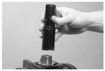
3. Install the stem adapter onto the valve stem.
