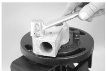
**13.** Install the locking lever onto the carriage bolt, as shown above. Do not tighten the lever fully at this time.
