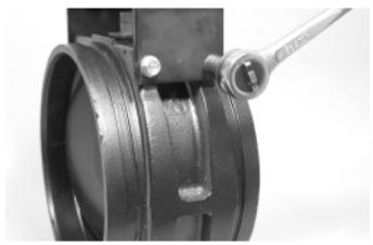
$\ensuremath{\textbf{1.}}$  Remove the four bolts that attach the valve bracket to the valve body.
