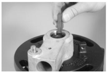
12. Install the key into the keyway in the stem adapter and handle's hub, as shown above.
