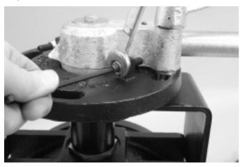
**18.** While holding the socket set screw in position, tighten the lock nut against the travel limit boss, as shown above. This sets the "FULL SHUT" travel stop.
