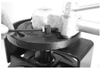
17. Make sure the valve disc is in the "SHUT" position. Turn the travel limit's socket set screw until it contacts the side of the handle's hub, as shown above.
