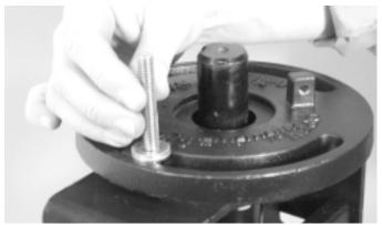
10. Insert two %-inch OD washers onto the carriage bolt.
