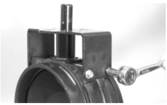
${\bf 5.}$  Re-install the valve bracket onto the valve body. Re-install and tighten the four bolts.
