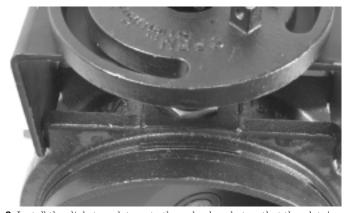
**6.** Install the dial stop plate onto the valve bracket so that the plate's holes align with the bracket's holes and the "OPEN" markings align with the valve inlet and outlet (refer to photos above).
