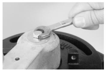
**14.** Secure the handle's hub assembly with the 1%-inch OD washer and the  $\frac{5}{16}$ -18 hex-head screw, as shown above.
