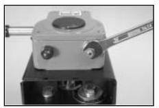
6. Tighten the hex lock nut (clockwise).
