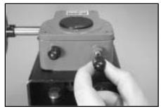
**1.** Remove the protective cap from the right side of the gear operator.
