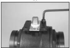
**4.** Using an allen wrench, remove the screw from the mounting plate of the valve.
