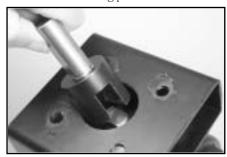
**2.** Install the stem adapter by positioning the flats of the stem adapter over the flats of the valve stem, as shown above.
