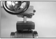
**5.** While supporting the drive hub, install the gear operator onto the stem adapter by positioning the flats of the drive hub over the flats of the stem adapter. Make sure the indicating arrow on top of the gear operator indicates the correct disc position.
