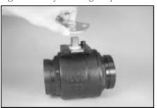
**3.** Remove the locking plate from the valve.
