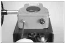
**5.** Using an allen wrench, tighten the internal set screw (clockwise) until it contacts the internal quadrant gear.
