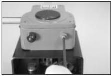
**3.** Using an allen wrench, loosen the internal set screw approximately three turns (counterclockwise).
