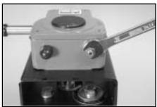
**2.** Loosen the hex lock nut (counterclockwise).
