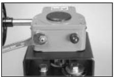
**2.** Loosen the hex lock nut (counterclockwise).
