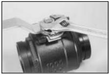
**1.** Remove the handle assembly nut from the lever handle, as shown above.
