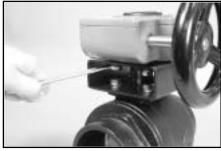
**6.** Place a lock washer onto each of the four hex-head screws, and hand-tighten the screws into the holes in the bracket and the gear operator. **NOTE:** Refer to the "Required Parts" chart on page 1 for the proper hexhead screw size and lock washer size.
