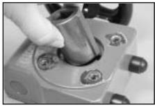
**4.** Insert the drive hub into the gear operator by aligning the key of the drive hub with the keyway in the gear operator, as shown above.
