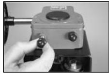
**1.** Remove the protective cap from the left side of the gear operator.
