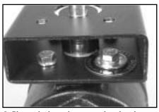
**3.** Place a lock washer onto a hex-head screw, and hand-tighten the screw into one of the holes in the bracket and the mounting plate of the valve. Repeat this procedure two more times. **NOTE:** Refer to the "Required Parts" chart on page 1 for the proper hexhead screw size and lock washer size.
