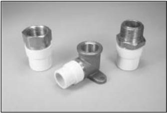
In addition, metal fittings with CPVC socket inserts can be used. For these fittings, the tubing is cemented directly into the socket by following the assembly procedures for an all-CPVC fitting.
