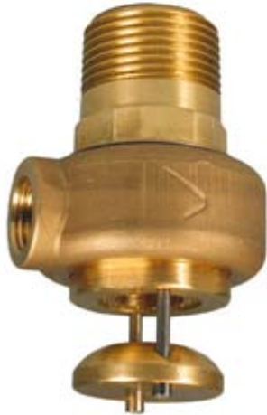
Series 953 Victaulic Vortex Emitter. Can be installed as pendent or sidewall. Can protect 2500 ft 3 / 70m 3 .
