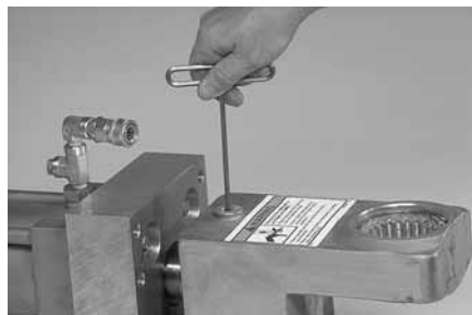
13. Turn the slide over, and loosen the set screw two full turns.
