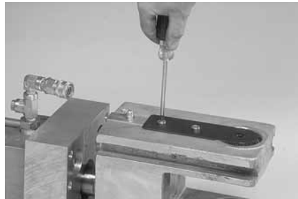
12. Remove the upper-shaft spring by removing the two screws.
