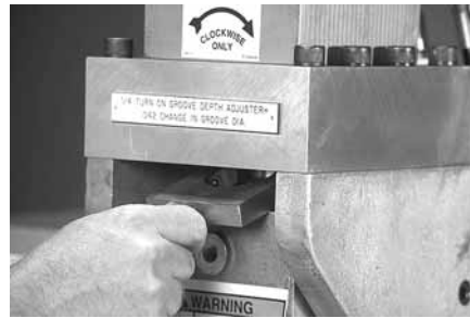
22. Snap the slide spacer into the tool, as shown above.
