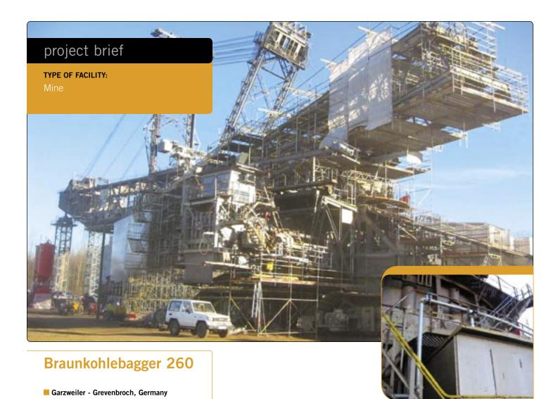
The Braunkohlebagger 260 Mine in Garzweiler - Grevenbroch, Germany needed a fire protection system for the retrofit of their 20 year-old brown coal excavator.
